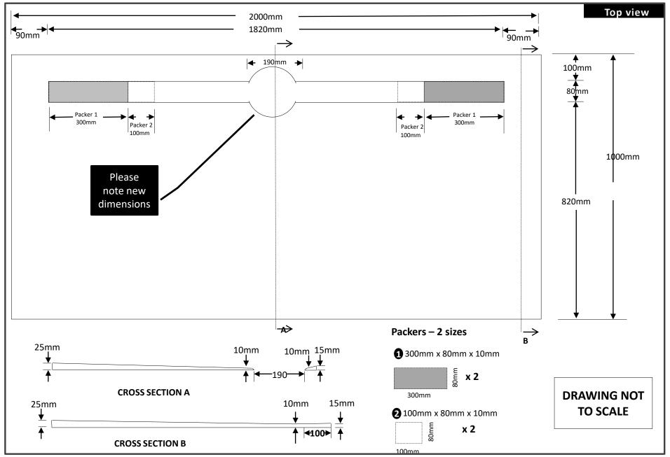
Channel drain – 1.0m x 2.0m Code: MXPST 1.0-2.0 TDLT
