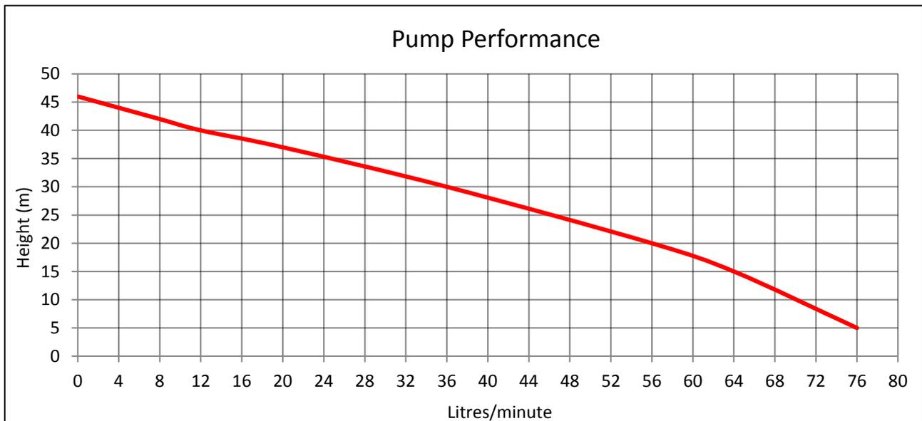
**NOTE:** The above Performance graph is measured at pump outlet and based on factory test conditions. Actual performance onsite may differ due to piping and fixture sizing and layout
