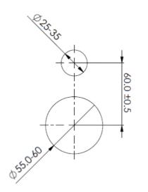
Note: The Mixer can be mounted 48mm to 73mm behind finished wall surface. Locate the correct position of the mixer by ensuring the "Hot" inlet, enters from the left. The top outlet is for the shower the bottom outlet for the bath. Ensure the diverter button is above the handle when the valve is fitted.
