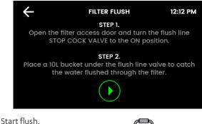
£ Approximately 10L of water will flow, for 2 minutes. FILTER FLUSH 12:12 PM RUNNING ..... Water is now being flushed through the filter. This process is automatic and will take 2 minutes. Press pause to pause filter flush.
