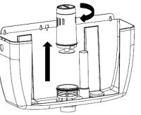
To remove the outlet valve turn the valve
