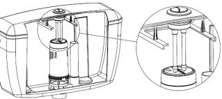
The button rods can be adjusted by screwing up or down the rod. After adjustment there should be 1 -2mm gap between the button rod and valve.
