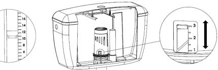
To adjust the half flush volume remove the valve and slide the float up or down.
