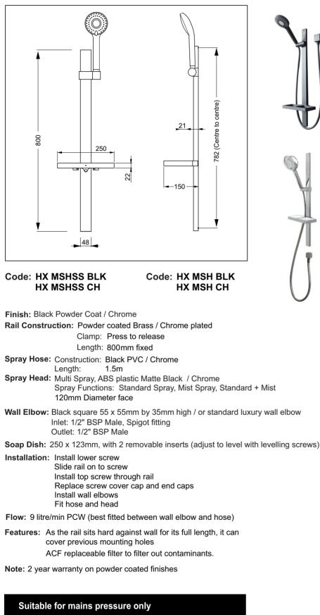
Recommended Operational Pressure Range: 150 - 600 kPa Maximum Operating Temp: 80°C Never to Exceed: 1000 kPa
