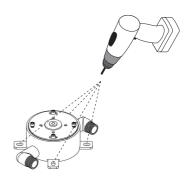
3 Wrap PTFE tape on the inlet elbows provided and screw them into the Underfloor Mounting Box.
