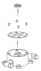
9 Align the copper pipes with the relevant hot & cold connector holes on the Underfloor Mounting Box. Fasten the fixing plate to the Underfloor Mounting Box.
