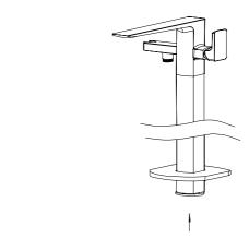
8 Fit the fixing plate onto the mounting plate (already attached to the Mixer Body in step 1).
