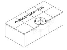
7 Remove the fixing plate, spirit level and blank cover caps.
