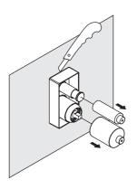
5 Install the flange & handle. It is recommended to apply a small bead of silicone behind the faceplate to prevent water entering the wall cavity.
