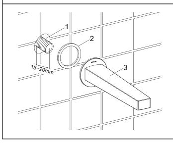
Apply tape or sealant to the G1/2" nipple(1, not provided) threads. Install the G1/2" nipple to extend 15~20mm beyond the finished wall.
