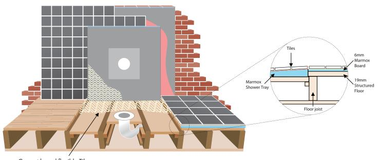
Cement based flexible Tile Adhesive (Classification C2)
