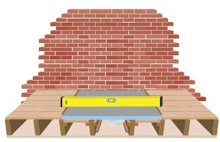
3 Use a flexible tile adhesive with 10mm notch trowel to fix the shower base to the floor. Place the shower base in position, apply downward pressure on the shower base and check for level.
