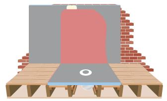
4 Apply any Branz approved water based waterproofing (non solvent based) to the entire surface of the shower base, flange and wall sheeting according to the manufacturer's recommendations.
