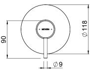
**CONSTRUCTION:** Stainless steel, brass and plastic CARTRIDGE TYPE: Ceramic CLASSIFICATION: Suitable for mains/high pressure only **INLET CONNECTIONS:** 1/2" BSP Male **OUTLET CONNECTIONS:** 1/2" BSP Male WORKING PRESSURE: 150 - 1000kPa
