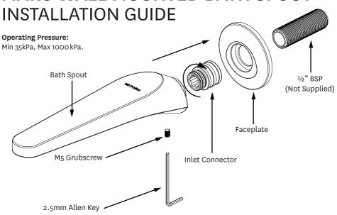
NOTE: Maximum hole diameter through wall for ½" BSP tube is 22mm.
