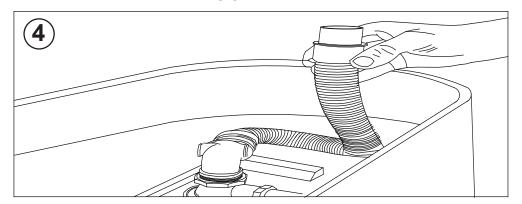
You can connect to it with a flexible drain pipe which enables you to tilt the bath up and move the bath into the required position. To avoid water retention in the trap the flexible pipe should have a continuous downward flow.
