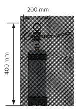
Secure cylinder vertically to a robust surface with the hook & loop strap and
