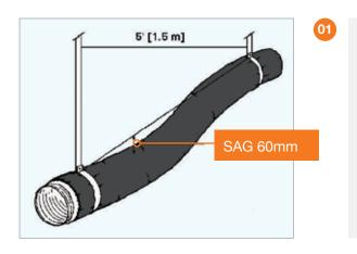
Flexible duct shall be supported at intervals, no greater distance than 1.5m. Maximum permissible sag is 60mm per metre of spacing between supports.
