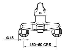
Supplied with aerator and flow director for spout CONSTRUCTION: Brass body outlet CARTRIDGE TYPE: Ceramic (SP033550) Removable flow restrictor on cold inlet CLASSIFICATION: Suitable for all pressure systems . 30mm extension available • New handle design **INLET CONNECTIONS:** 1/2 " BSP Female WORKING PRESSURE: 35 - 1000kPa DIMENSIONS FOR FITTING: 150±50mm distance between connectors **OPERATING TEMPERATURE:** 5 °C - 80 °C WATER FLOW RATE: 12.0 l/m FU2080CP2 Chrome
