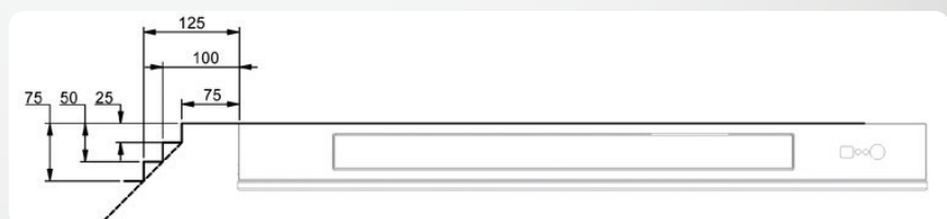
Arriva 752 surround clearances
