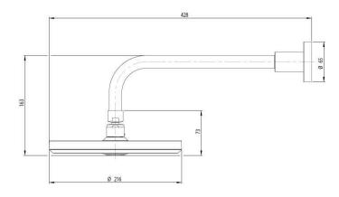
CONSTRUCTION: 320mm wall mounted arm CLASSIFICATION: Suitable for all pressure systems WORKING PRESSURE: 35 - 500kPa INLET CONNECTION: 1/2" BSP female OPERATING TEMPERATURE: 5 °C - 70 °C WATERFLOW RATE: 9.0 l/m
