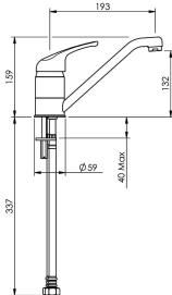
CONSTRUCTION: Brass body CARTRIDGE TYPE: SP033510 ceramic cartridge CLASSIFICATION: Suitable for all presures INLET CONNECTIONS: 1/2 " BSP WORKING PRESSURE: 35 - 1000kPa DIMENSIONS FOR FITTING: 35mm diameter hole OPERATING TEMPERATURE: 5 °C - 80 °C WATER FLOW RATE: 9.0 l/m low pressure - 8.0 l/m high pressure
