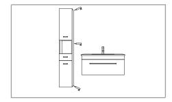
Materials used for the construction of this unit are water resistant and not waterproof. A bead of sealant (specifically formulated for bathrooms) must be used to seal all edges where water penetration can occur. i.e. Between the cabinet and the wall. Take care to dry any spillage or leakage of water onto or into the cabinet during installation.
